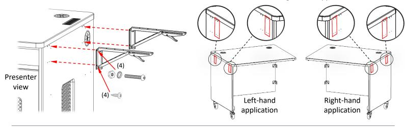
Once brackets are installed, continue to fasten to the shelf by driving the 5/8" screws into pre-drilled holes. 2
